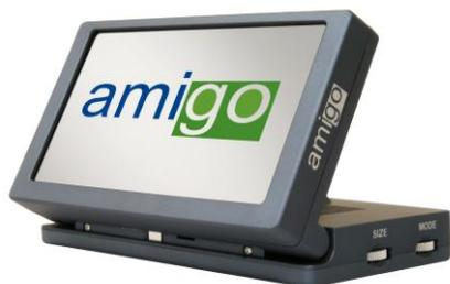
Amigo is a truly portable desktop magnifier. Optimal viewing is achieved with a tilting 6.5 inch viewing screen. Amigo provides 3.5 to 14x digital magnification and the lightest weight in its class. Amigo is battery operated and can be taken anywhere.
